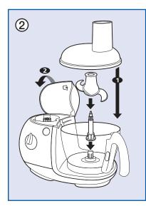
MIXING/BLENDING/CHOPPING/ KNEADING - (DIAGRAM 2) Accessories used (depending
